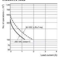
A current of 0.15 A max. can be switched at 125 VDC (cosφ=1) and current of 0.1 A max. can be switched if L/R=7 ms. In both cases, a life of 100,000 operations can be expected.
